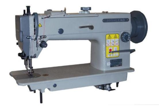
TECHNICAL DATA intended for heavy materials max. sewing speed 2000c / min stitch length 0-10mm manual foot lifting 6mm, knee 16mm central lubrication ORGAN DPX17 needle type bead travel (differential) 2 - 5mm change of the differential with a lock knob height of the teeth 1mm 260 x 125mm working space Power Max AH clutch or energy-saving motor 2. Overlock Highlead GM288 - 501 for overcasting medium fabrics, 5-thread, 4.8mm gauge between the needles.
